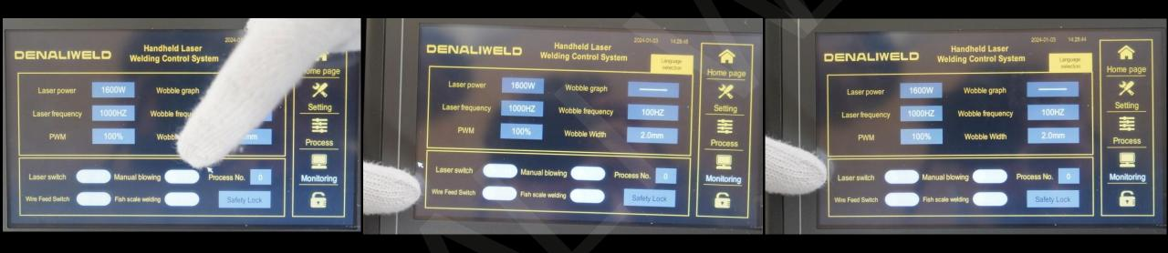
Toggle gas manual to on position to ensure gas flow. Then turn off (you will audibly hear this)
