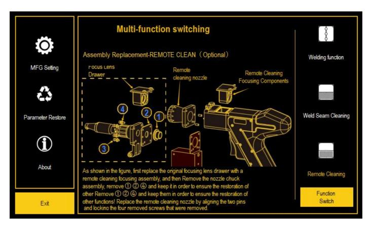
• Function Switch: select required function and click "Function Switch" to enter sub-interface of selected function.
