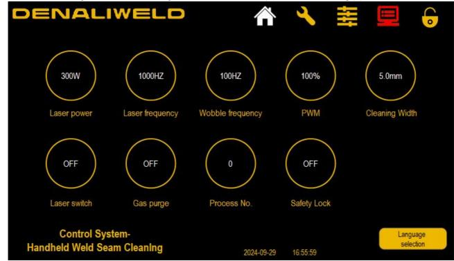
• Select the weld cleaning function, and modify the process parameters according to the process requirements.
