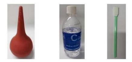
If there is dust on the lens: firstly using the aurilave ball to blow the dust off, then clean the lens carefully with a dry cotton swab, without using force.
