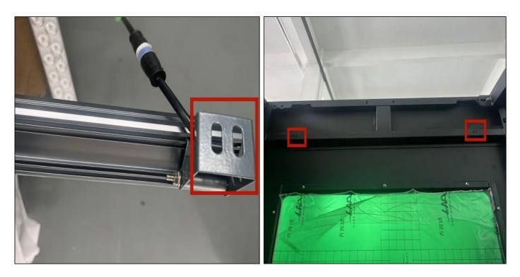
The diagram below shows, where the lamp post connection begin, The front and back sides are fitted with lamp posts, four in total, connected to each other as in the picture below.
