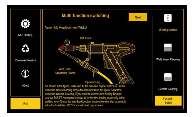
• Weld Seam Cleaning: show assembly replacement diagram.
