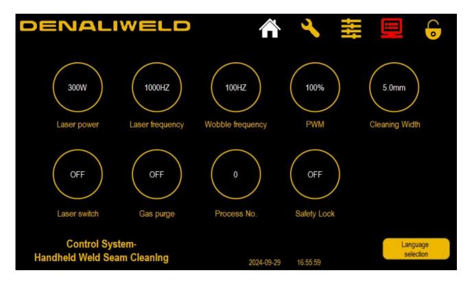
• Select the weld cleaning function, and modify the process parameters according to the process requirements.
