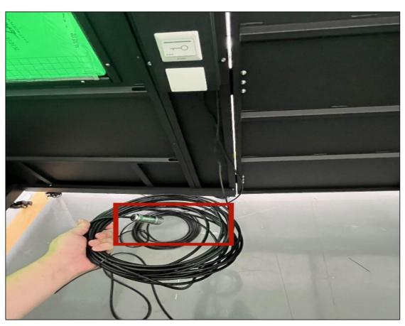
The following diagram shows the 220-volt power connection cables that are supplied to the lampposts, access control unit.
