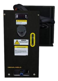
The cooler is responsible for maintaining a constant water temperature, which removes the heat of the laser source and the welding head. All parameters of the radiator module have been set before leaving the factory. Do not change the settings if not authorized by the supplier. Only the purified water should be poured into the chiller and the purified water should be changed every month.
